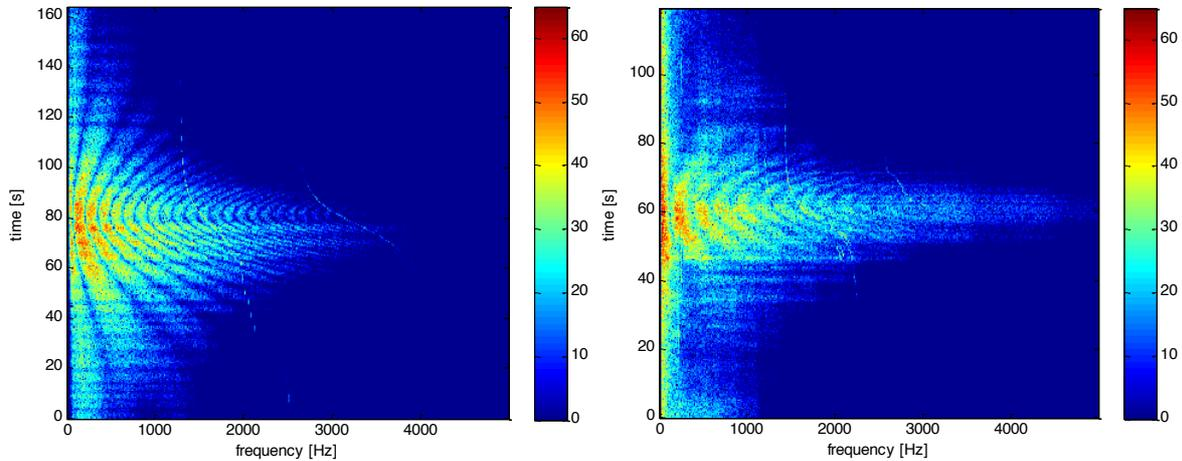
**Figure 2:** Noise fingerprint for landing: (left) ANCS synthesis, (right) noise recording
