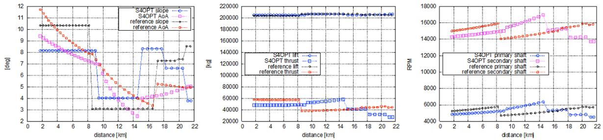
**Figure 5:** AC2 take-off: slope and aircraft attitude & lift, thrust and shafts' RPM for the optimal solution.
