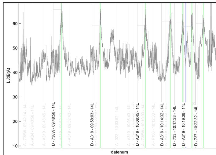
**Figure 4:** Example of found events in the SPL-Log (green lines) and the assigned flights from the schedule (black lines with text). The grey lines with text are the remaining events from the schedule. The meaning of the texts: “[D]eparture or [A]pproach – Aircraft type – Time – Runway”.
