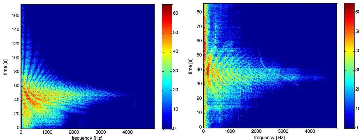
**Figure 3:** Noise fingerprint for take-off: (left) ANCS synthesis, (right) noise recording
